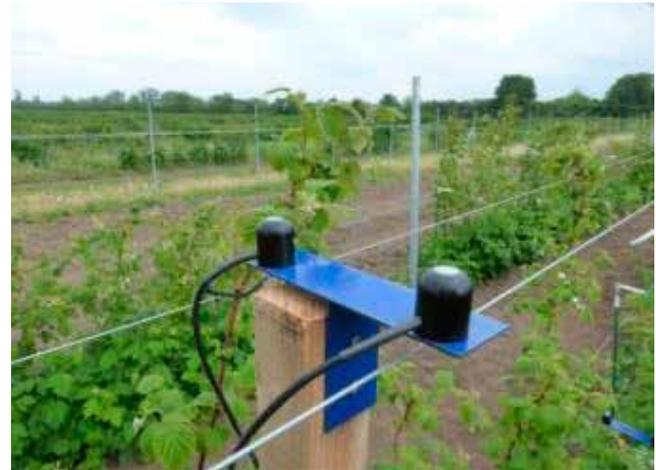
Figure 3: PYR Apogee SP-110 360-1120 [nm] and PAR Apogee SQ-100 380-720 [nm]
