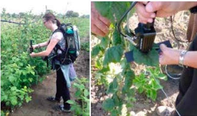
Figure 6: ASD FieldSpec 3 MAX with PlanProbe sensor head and a Cubert snapshot camera
