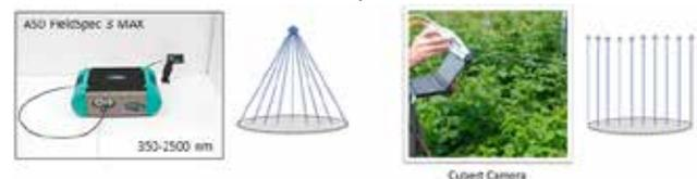
Figure 5: Operation principle of ASD FieldSpec 3 MAX and Cubert snapshot camera
