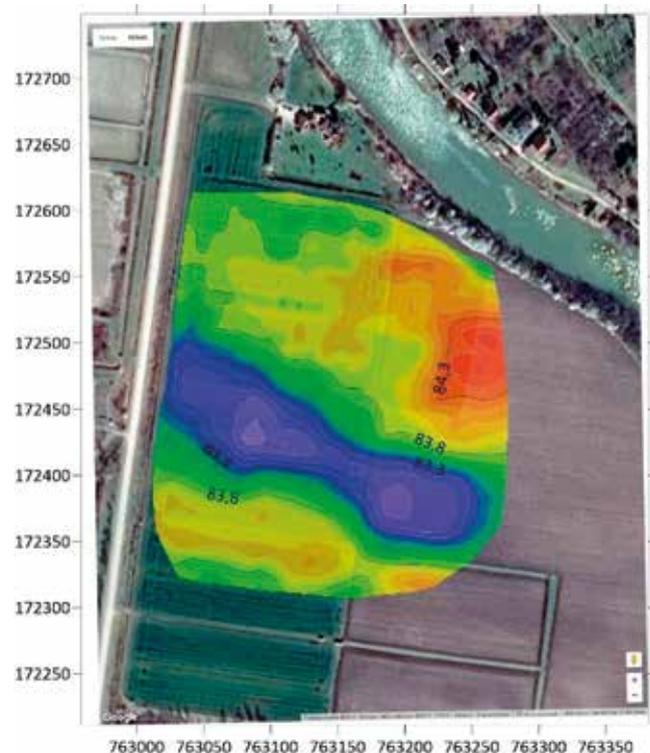
Figure 1.: Heterogeneity of relief under a precision centre pivot. Blue colour represents low and red represents high relief.
